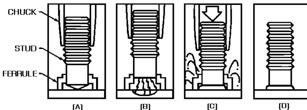
**Figure A3** - The Welding Process
