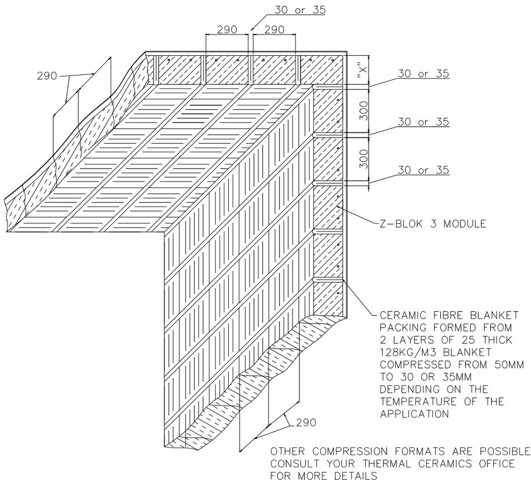
**Figure 3 - Typical Z-Blok 3 Module Lining**
