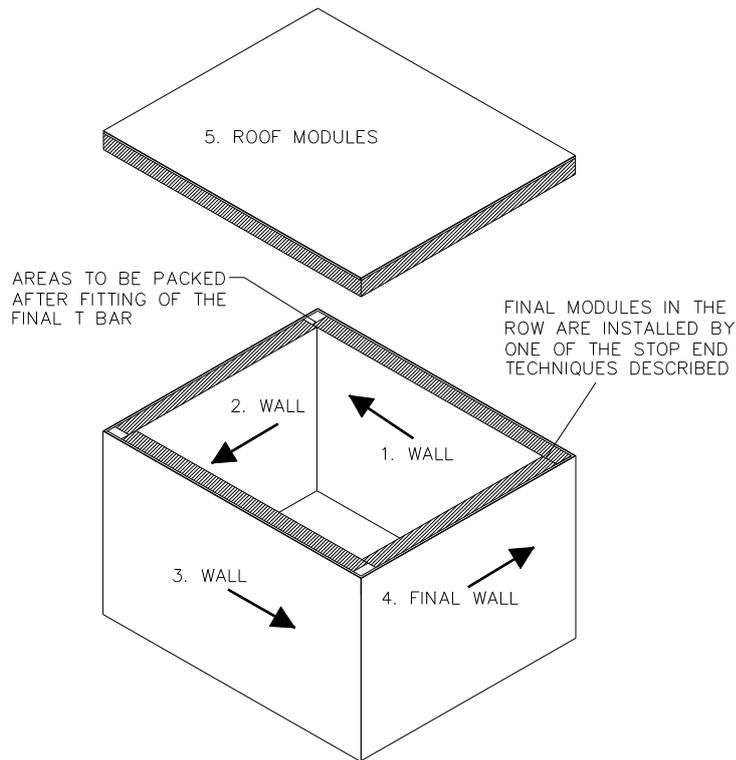
**Figure 6 - Installation Sequence for a Four Fixed Wall and Roof Application.**
