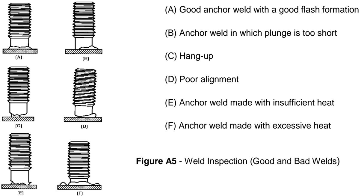
**Figure A5** - Weld Inspection (Good and Bad Welds)
