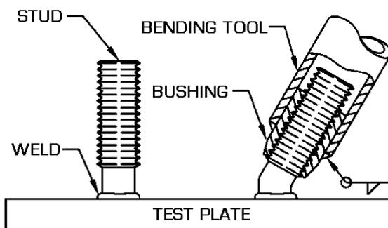
**Figure A6** - Bend Test
