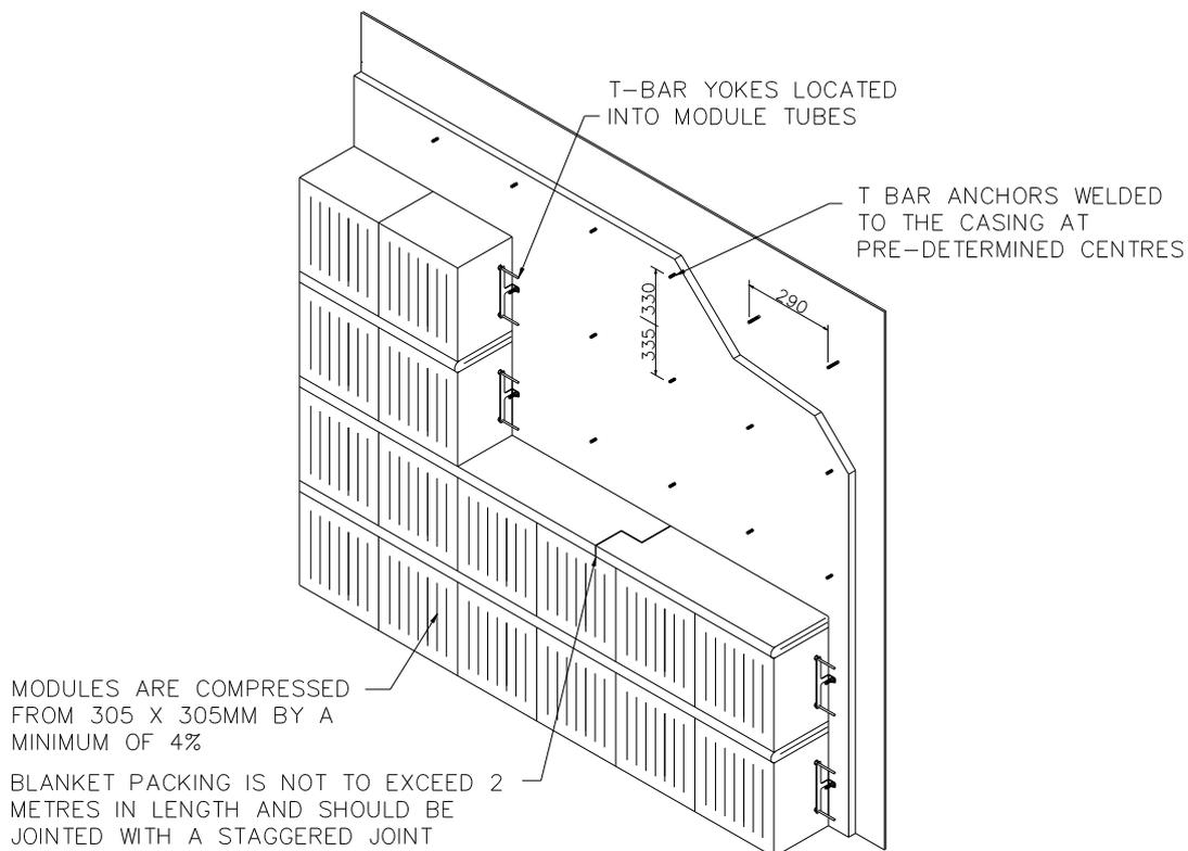
**Figure 2 - Typical Z-Blok 3 Module Lining and Anchor Layout**
