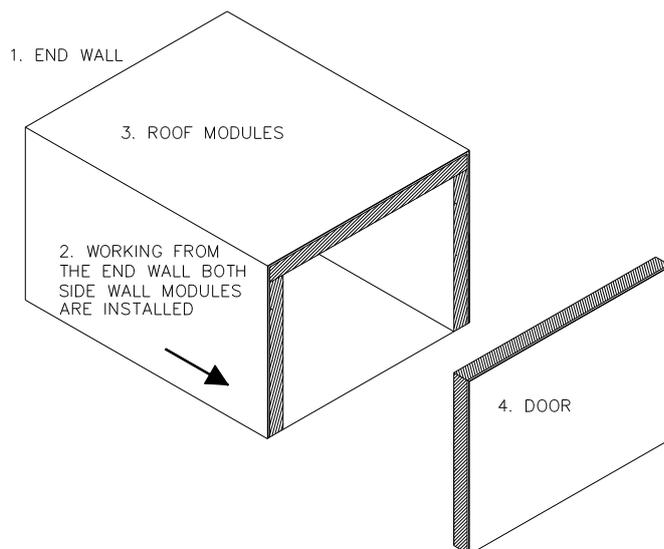
**Figure 5** - Installation Sequence for a Three Fixed Wall, Roof and Separate Door Application.
