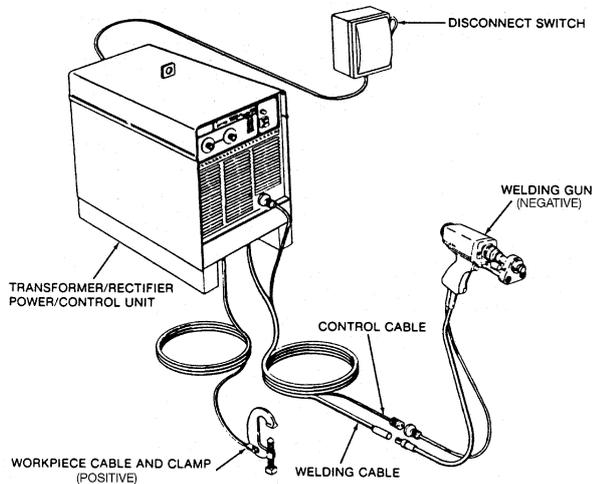
**Figure A2** - Equipment Set-up with Power Source and Control Box Combined
