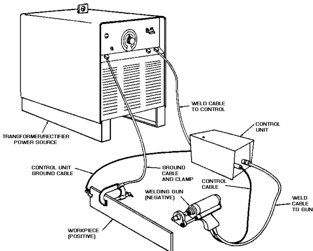
**Figure A1** - Equipment Set-up with Separate Power Source and Control Box
