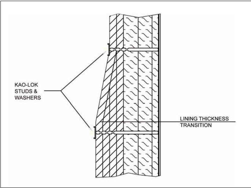
Figure 10 - Typical Lining Thickness Transition Detail
