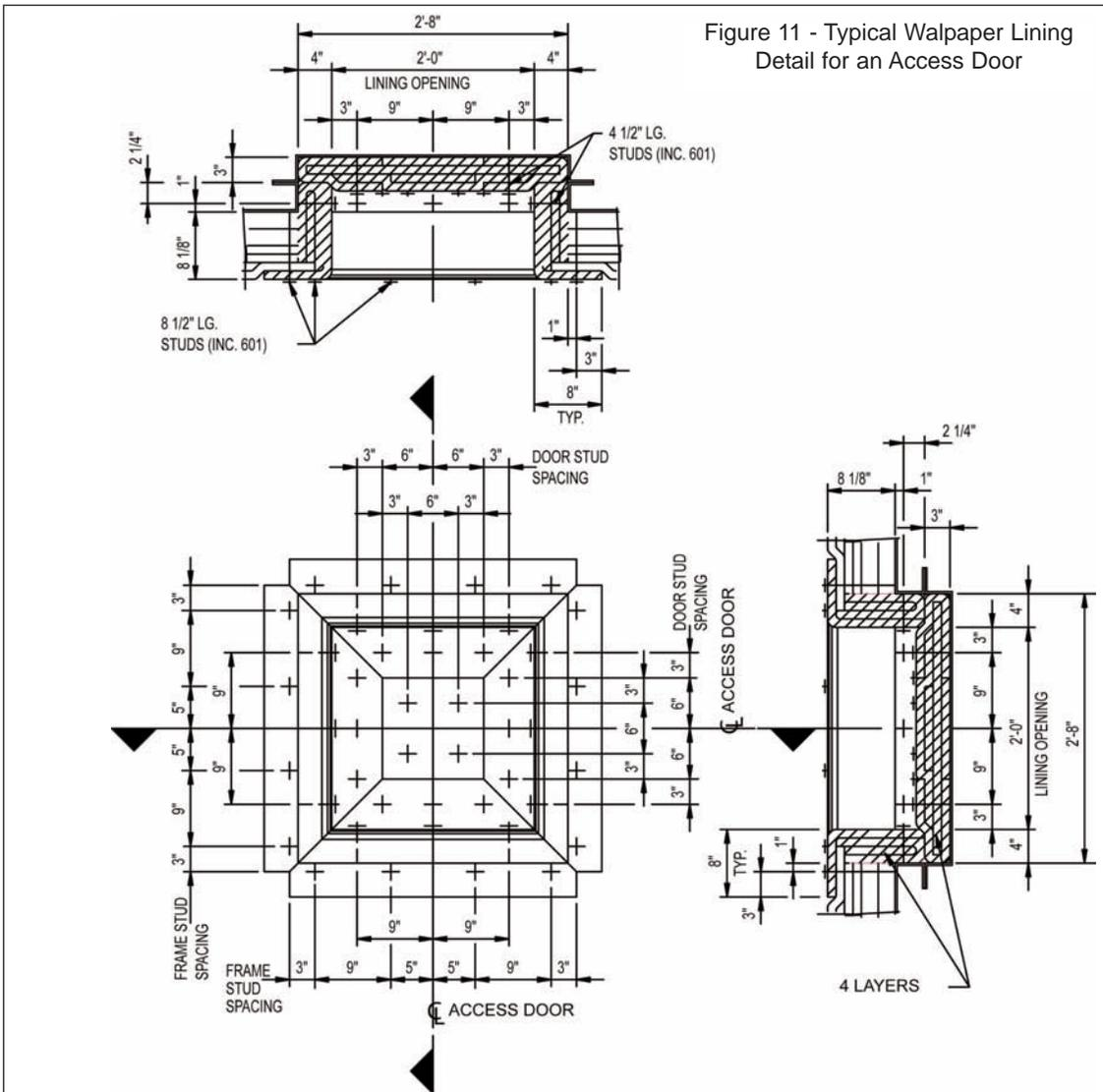
Figure 11 - Typical Wallpaper Lining Detail for an Access Door
