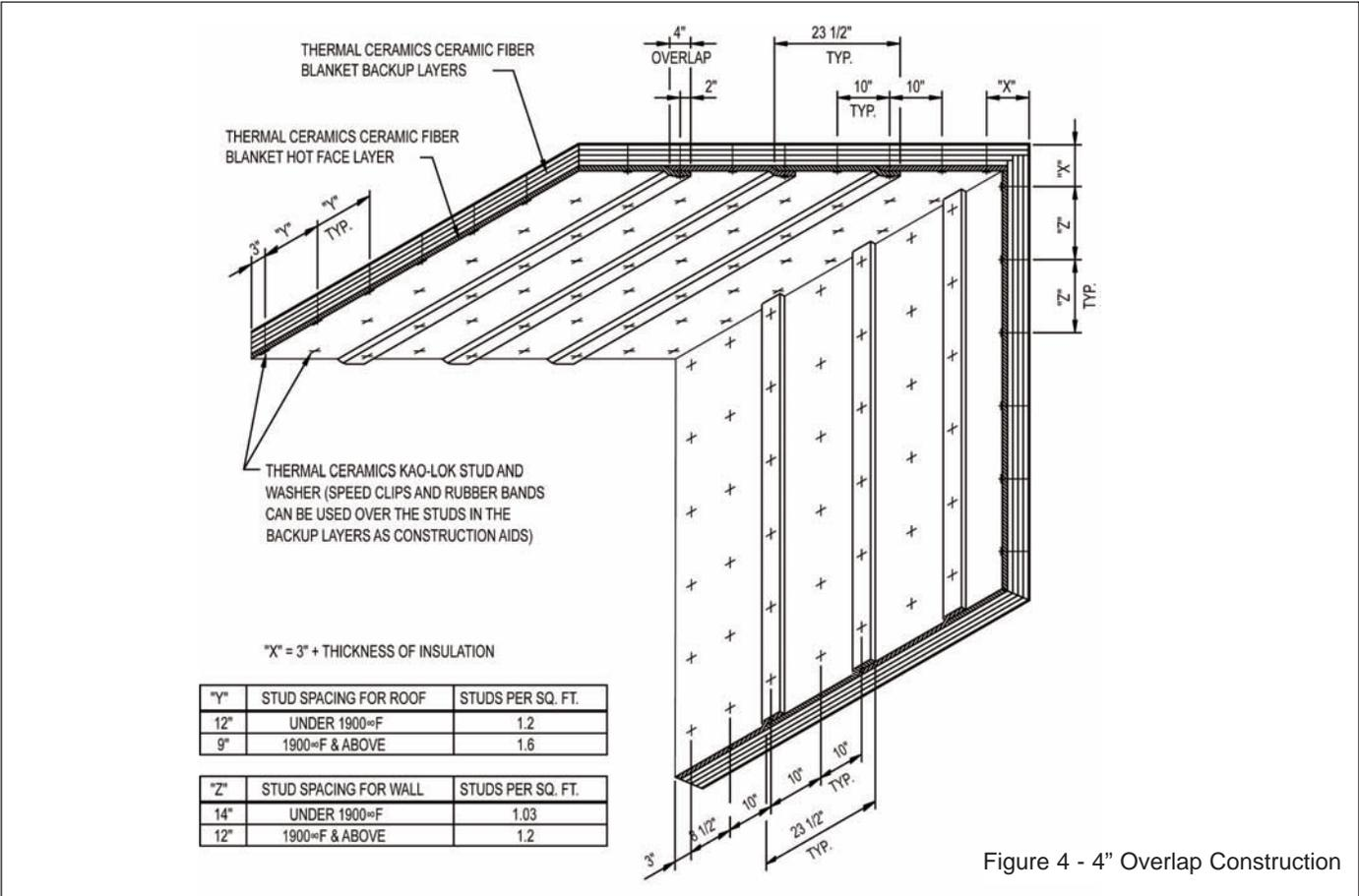
Figure 4 - 4" Overlap Construction
