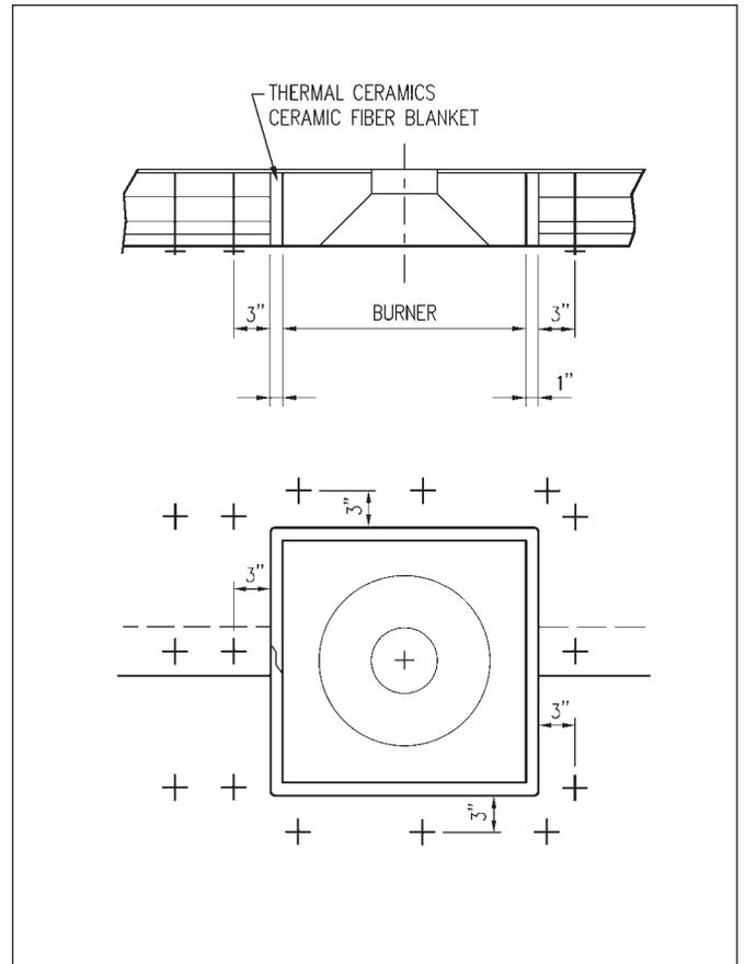
Figure 9 - Burner Wrap
