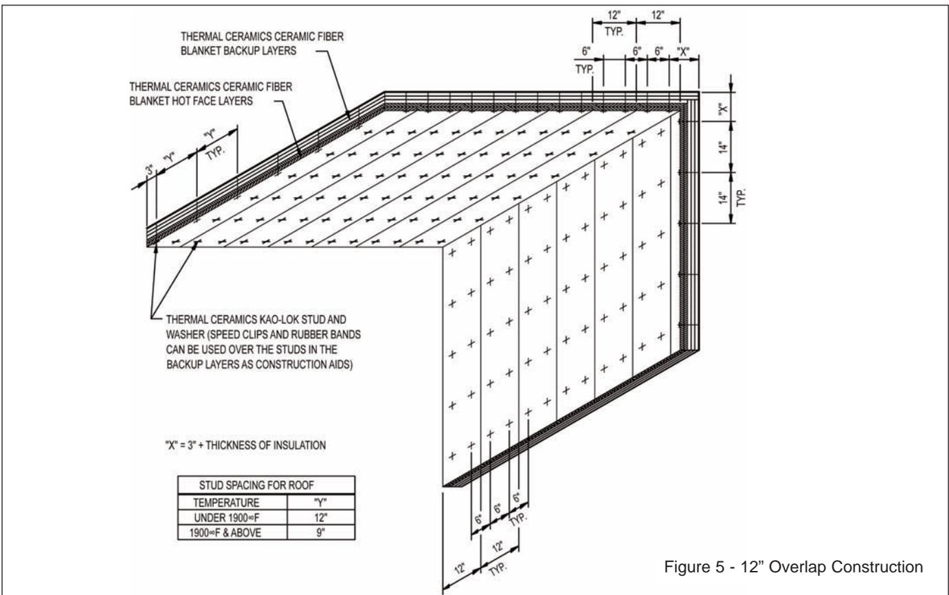
Figure 5 - 12" Overlap Construction
