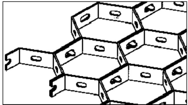
Figure 14 - Hexmesh Anchoring System
