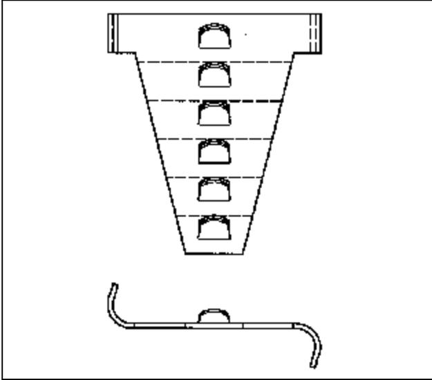
Figure 15 - S-Bar Anchoring System
